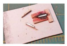
Figure 40: The assembly jig for the floor board hangers.
