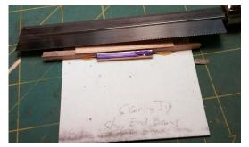
Figure 37: One of the end beams in the scoring jig.
