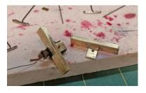
Figure 39: Coupler mounting plates were made of 0.032" by 4" brass strip. They were drilled and tapped, as seen here, and fitted with couplers and draft boxes.
