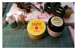
Figure 34: These are the solder flux products used for this installment. From left to right: Tix Flux and Anti Flux, Rubyfluid, and Fry's.
